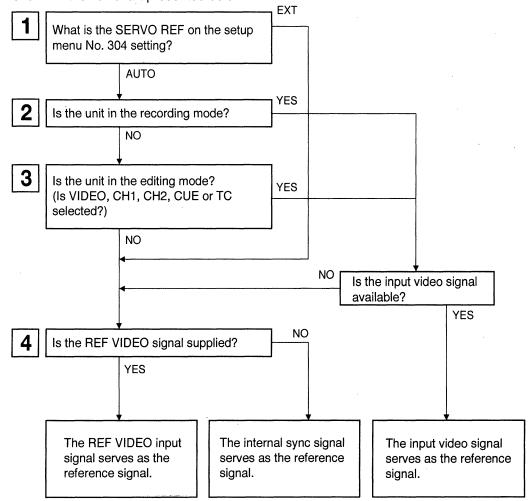
The servo reference signal is switched as shown in the tables below depending on the servo reference setting, deck mode and what input signal is available. When the mode is transferred to editing or recording/playback, the image may be disturbed and the transfer may be delayed if the references during playback and recording do not match.
